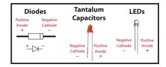
Check and make sure the components with a positive and negative side are installed correctly. Check the instructions if you're unsure about the correct orientation of these parts. Orientation is covered in the instructions. Also, if it's a "Plus Mod" with an adapter assembly, make sure the chip sockets (cradles that holds opamps) are soldered to the adapter pcb and that the orientation of the opamps are correct.
